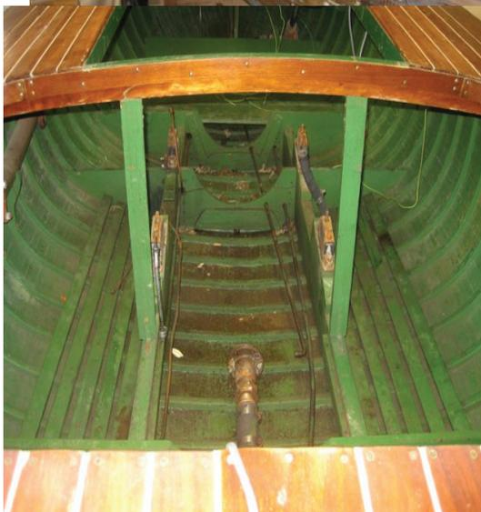
*The metal rub rails came with half round pieces of wood beneath them. These were dry, cracked, and completely missing in areas. They were re-fabricated and installed prior to varnishing.*
