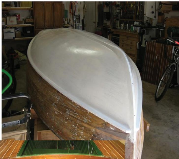
*When the boat was turned again, a fillet was added to the top side of the rails with a strip of glass following. After fairing the topsides a layer of fiberglass was applied, followed by two-part primer and paint.*
