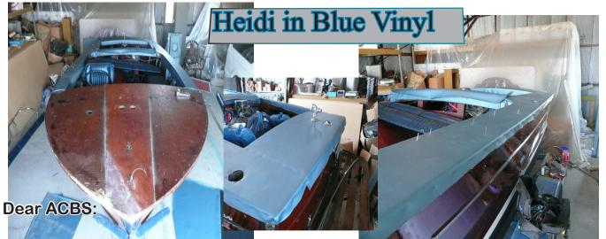
These are some of the photos of my vinyl deck replacement. I used either Monel or SS staples and was working on my second thousand when it was completed. I fitted the old vinyl over the new decking and matched up the existing holes in the vinyl with the holes in the underlying wood to replace the deck hardware. Some judicious poking around with pins located the previous holes.
